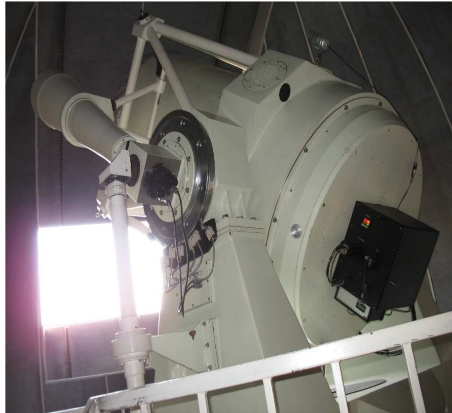
1 Meter SLR telescope made by Shanghai Observatory
