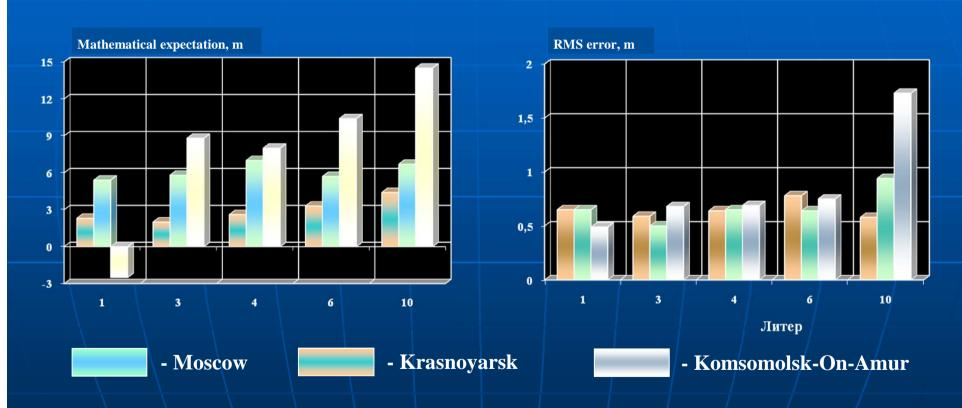
**Result:** calibration accuracy of one-way measurement systems is ensured at decimeter level – For GMS this error is less than 0.5 m (RMS)
