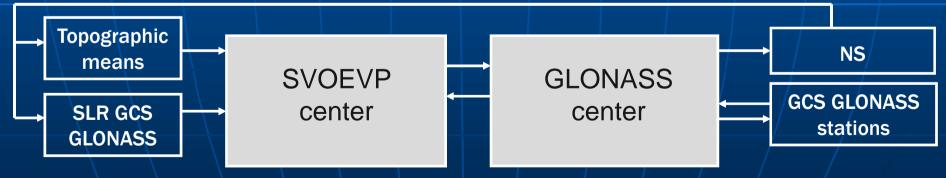
First time in Russia there was created a System for check of accuracy of transfer of initial reference frame by GLONASS navigation field.
