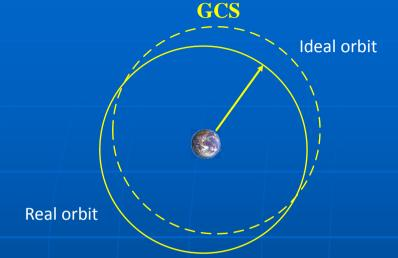
Shift along Z axis at the pericentre of GLONASS near-circular orbit over Russian territory leads to fixation of the determined orbit below optimal one, rise of apogee part of the orbit and error in calculation of eccentricity.
