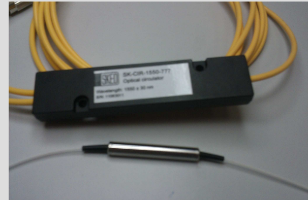
Optical Circulator and optical isolator
