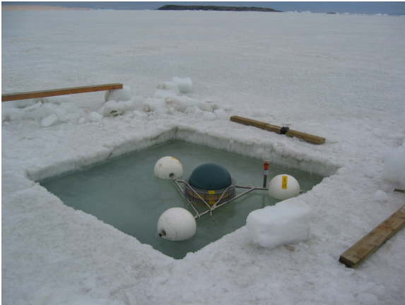
Fig. 1: The UTas GPS buoy
