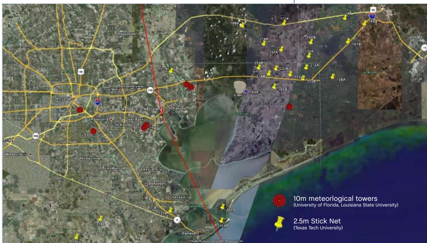
Figure 6 The track of Hurricane Ike and the locations of the meteorological instrument platforms on a Google Earth map.
