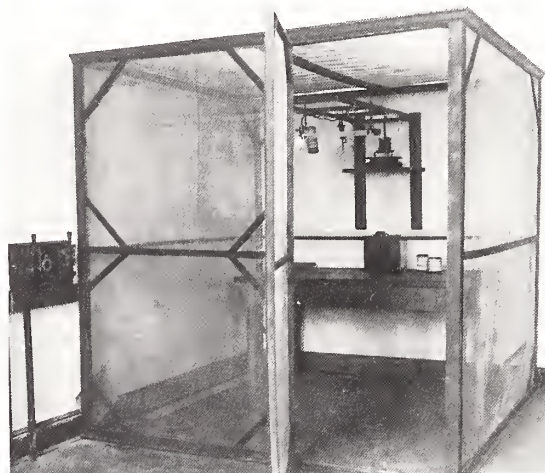
An early shielded room or "cage" developed by the Radio Section. The first attempt at shielding was in 1917 with considerable success in minimizing the strong signals of NAA, the powerful Navy station across the Potomac in Arlington, Va.
