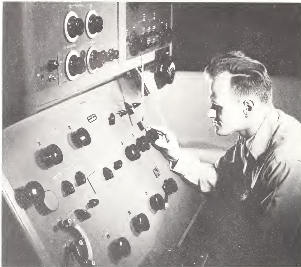
This photograph in "Rembrandt lighting" taken of Thomas Zapf during second year of operation of the Electronic Calibration Center (1959). A calibration is being performed with a highly refined type of capacitance bridge developed by the combined effort of two instrument manufacturers.
