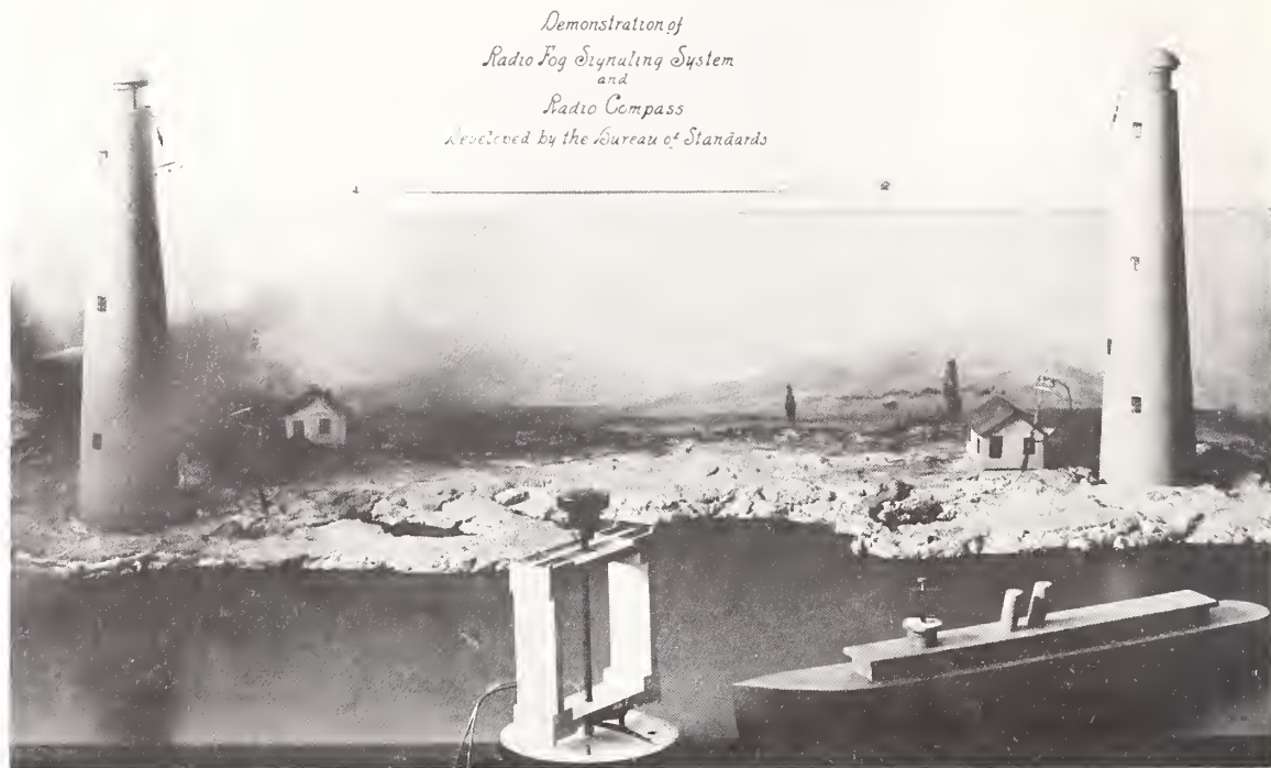
Model prepared by Radio Section to demonstrate a radio "fog signaling" system—using a direction finder (or radio compass) to determine position of ship by triangulation method. Radio direction bearings are taken on two land-based transmitters.
