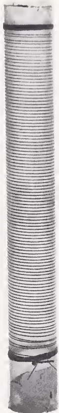
Early form of the electrical hygrometer developed by Dunmore for use on radiosondes to determine relative humidity. Dunmore experimented with this device for more than a decade, bringing about many changes and improvements. In principle, the electric resistance of a film of lithium chloride indicates relative humidity over a wide range. Several patents came from this device and it is used quite extensively today.
