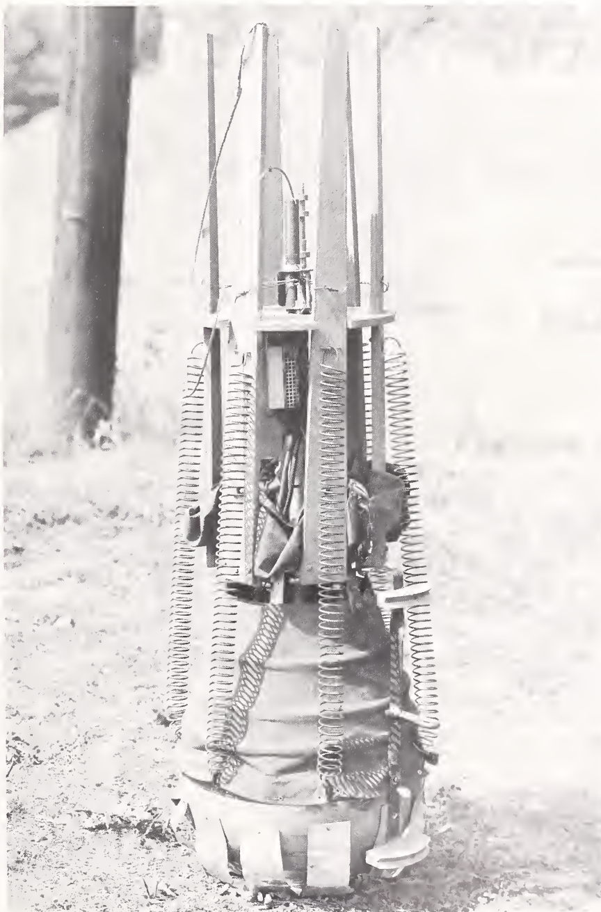
Automatic weather station designed for descent by parachute from airplane to observe weather conditions in remote sectors of enemy territory. The sensing equipment and radio transmitter were patterned after the radiosonde that had its initial development about 7 years earlier in the Radio Section. The six "legs" of "Grasshopper" (the name selected after initial development) are shown in their folded position for carrying in bomb rack.
