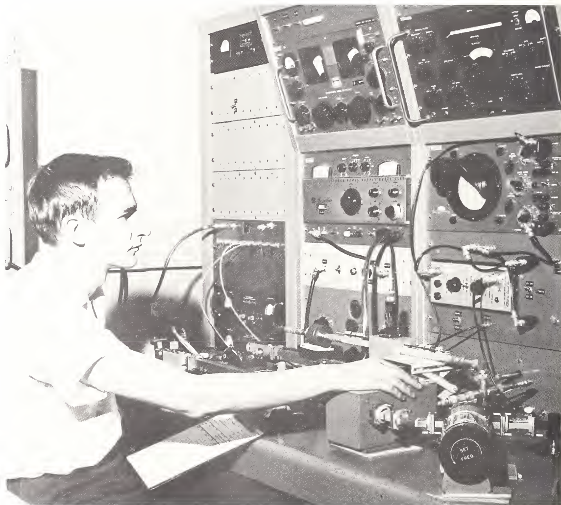
Norman Abshire of the Electronic Calibration Center calibrating a cavity-type wavemeter at microwave frequencies in 1963. By this time, 18 years after the first microwave frequency standard had been developed by the Bureau, the upper frequency limit of the standard had reached 90 GHz. Limits of uncertainty of measurement were about 2 parts in 10^6 .
