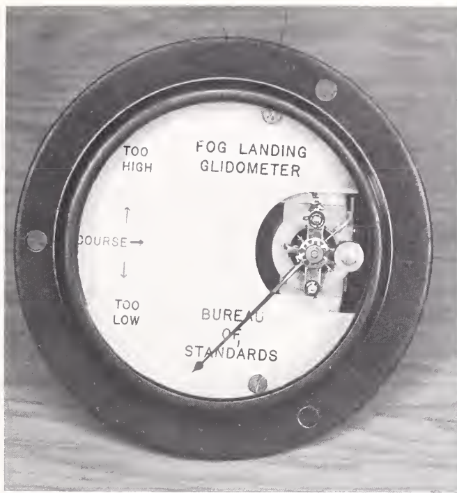
Early form of landing beam indicator. Used by pilot to follow proper glide angle in a blind landing.
