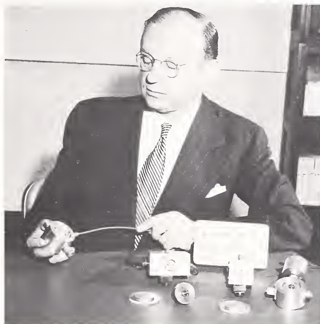
Myron Selby in 1956 observes his recent development of the micropotentiometer for accurate measurement of RF voltage at frequencies ranging up to 1000 MHz. At right is rack of interchangeable disc resistor assemblies that give the "micropot" a range from 1 microvolt to 0.1 volt.
