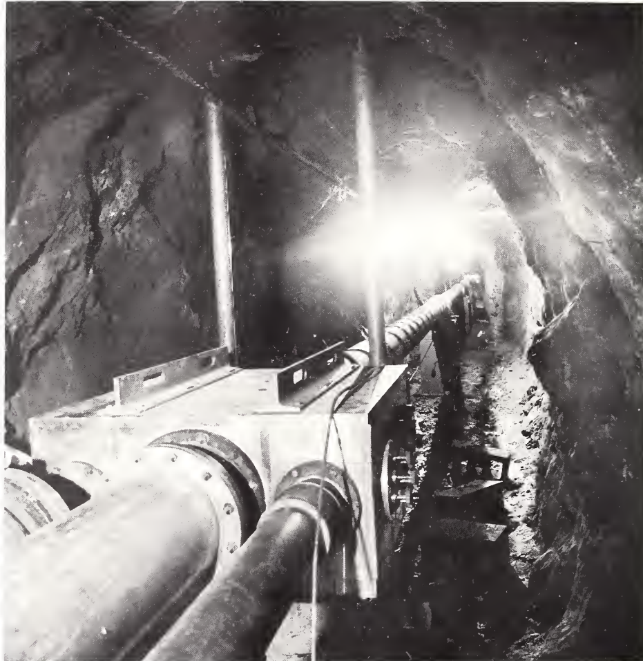
A laser interferometer, 30 m long, in the Poorman's Mine (an abandoned gold mine in the mountains west of Boulder) served as a laser-seismograph to measure vibrations in the Earth's crust.
