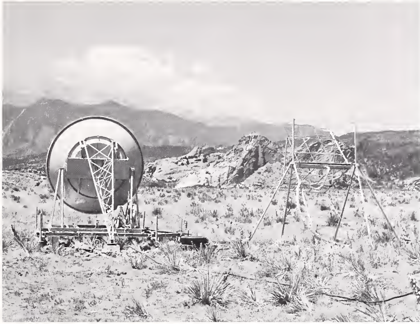
Portable receiving equipment used in line-of-sight propagation path between Pikes Peak (left center) and the Garden of the Gods, Colorado Springs, Colo. This path (approximately 10 miles) offered an excellent opportunity to observe both ends of the path and changes, such as cloud formations, taking place in the intervening distance.
