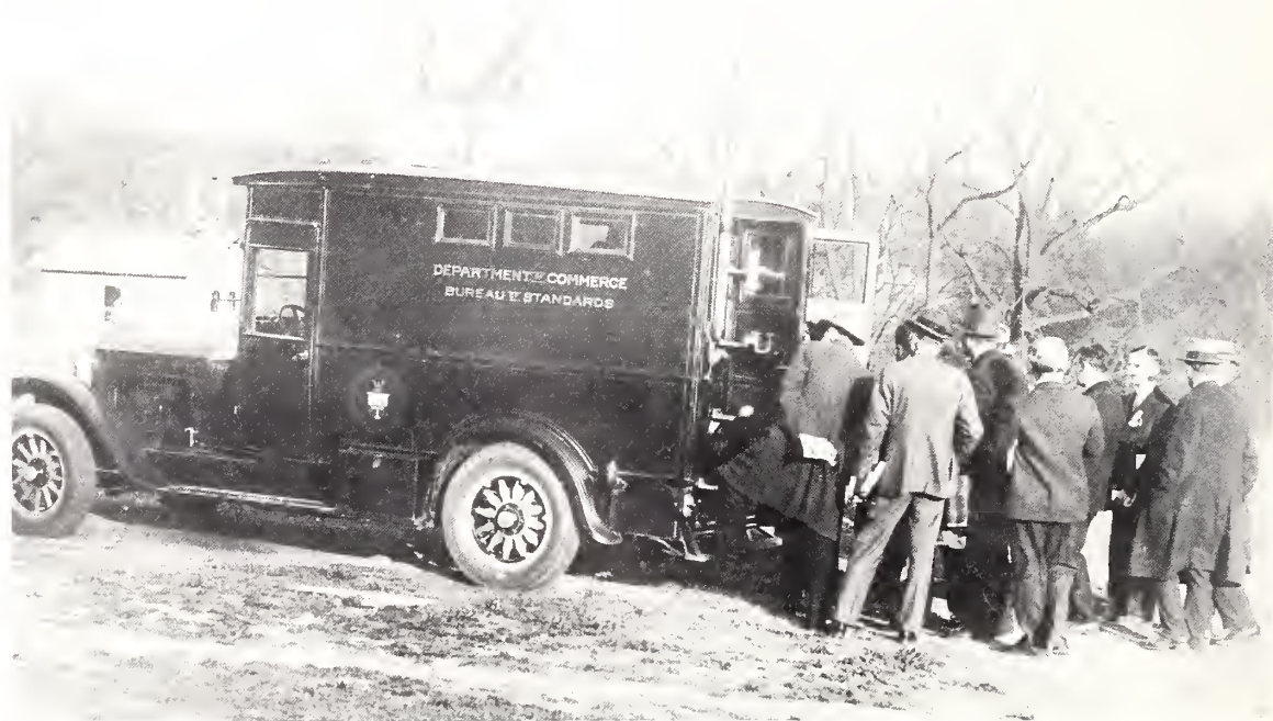
Delegates to International Radio Conference, Washington, D.C. in fall of 1927, inspecting the mobile radio laboratory at the Bureau of Standards. The laboratory truck was used in various parts of the country to make field measurements of fading and intensity of radio signals.
