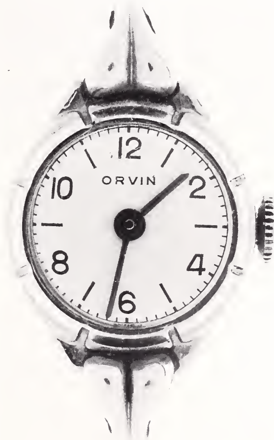
This lady's wrist watch used with the Model C-1 ionosonde (only one instrument constructed) that was developed in 1945. There was no scale of frequency or height on the ionogram, and time of sweep and time of day were recorded for each ionogram by photographing the watch (alongside of tape record). The setting of 1:32, on this watch of historical interest, is that on a published ionogram.
