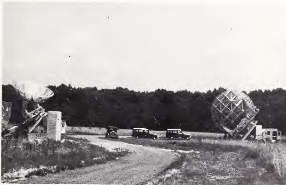
Two of the three Würzburg (Giant) antennas installed at the Sterling, Va., field station, northwest of Washington, D.C. The 25-foot diameter paraboloidal "dish" antennas were developed by the Germans during World War II for long-range search radars. The antennas were brought to Sterling for a study of solar radio noise.
