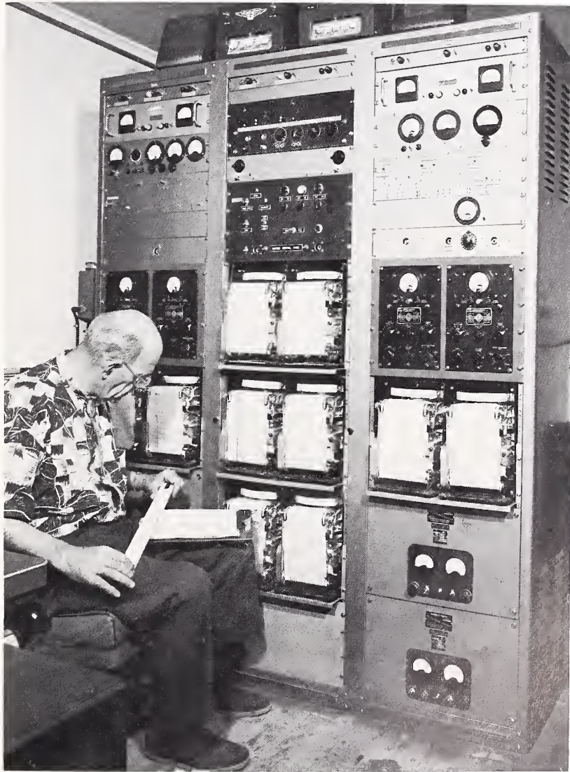
Recording equipment in the Solar Patrol building on Gunbarrel Hill, northeast of Boulder, Colo. Radio waves received from the Sun at two frequencies (167 and 470 MHz) are amplified and recorded on continuous charts. Wesley I. Nodine is the observer.
