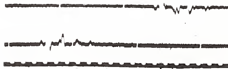
Typical 1410 kc pattern as received at Kensington, Md., during night period, (3:33 A.M., April 13, 1930). Note small peak, large peak, and then series of small peaks.
