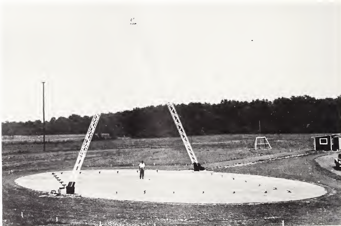
Model antenna range at the Sterling field station near Washington, D.C. The site is now occupied by Dulles International Airport. Designed to measure antenna radiation patterns in the vertical plane, the antenna is placed at the center of an oval-shaped metallic ground plane. The inverted V-frame of plywood carries a self-contained target transmitter at the apex and can be moved through a 180° arc. Photo taken in July 1951 shows V-frame at the 90° position. Using the model technique, this model permits measurements to be made in the frequency range of 60 to 1500 MHz, simulating antennas that operate in the range of 1 to 25 MHz.
