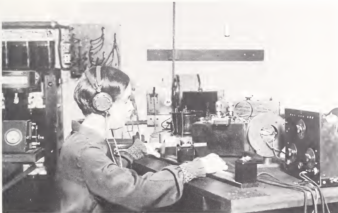
In the mid-1920's quartz plates, used as frequency standards, were calibrated by beat-note comparison with a high harmonic (from a harmonic amplifier) of a calibrated tuning fork. Miss Grace Hazen is using a sonometer (stretched steel wire calibrated at audio frequencies) to determine frequency of beat note.
