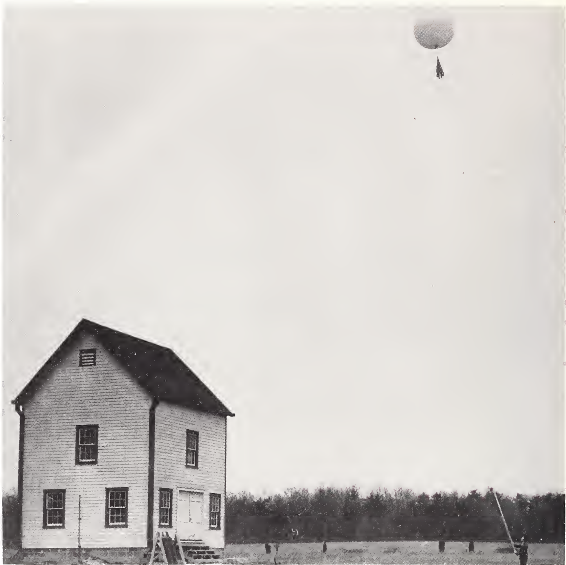
Launching a balloon-borne re-emitter (receiver-transmitter) at the Beltsville, Md. field station to determine wind speed and direction by a phase-variation method. Re-emitter package held on pole to prepare for launching (package can be seen at treetop line). The parachute will safely lower the re-emitter after bursting of balloon at high altitude. Building houses the directional antenna and ground-based electronic equipment. A project of the early 1940's.
