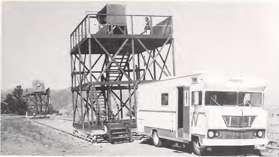
Outdoor 50-meter antenna extrapolation range located at edge of mesa at rear of the Boulder Laboratories site. On-axis antenna gain is measured by using two antennas, each mounted on its own movable tower. Towers can be separated at known distances by moving on accurately aligned rails. Measurements are recorded in the van and a computer analyzes the observations.
