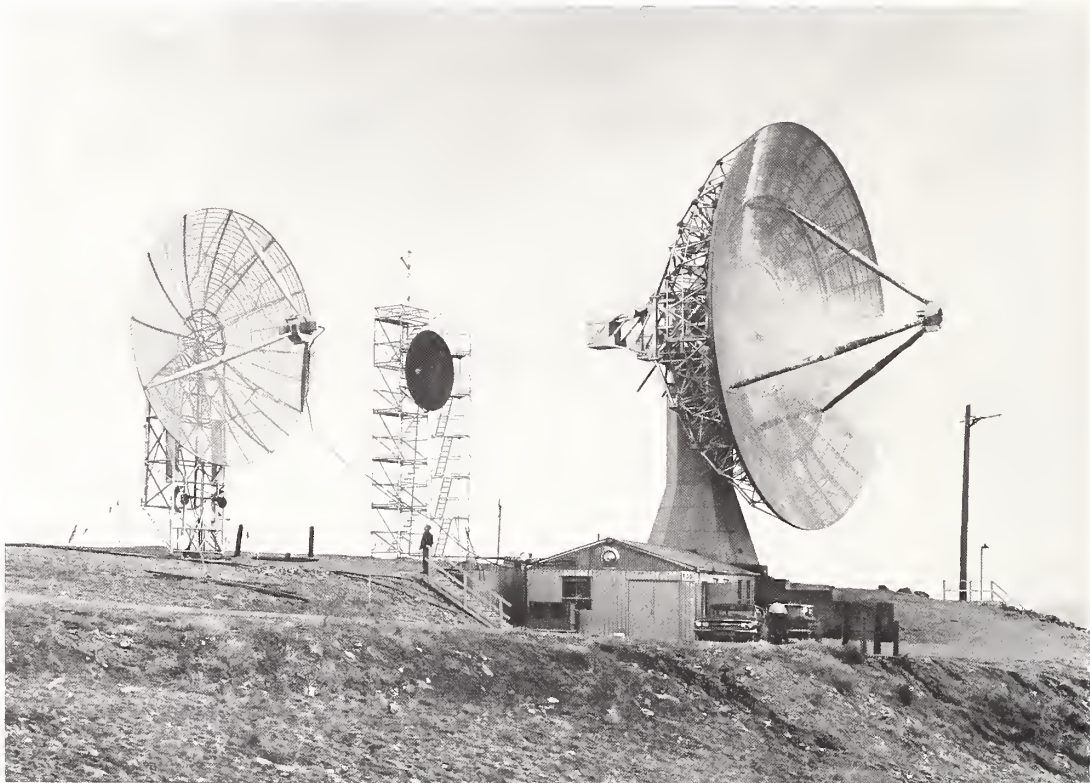
Antenna array at the CRPL Table Mountain field site north of Boulder, including a pair of 60-foot-diameter parabolic antennas. The antennas shown here were located at one corner of the almost level surface of a mesa (approximately 1 mile \times 2 miles) (Table Mountain) which formed the field site.
