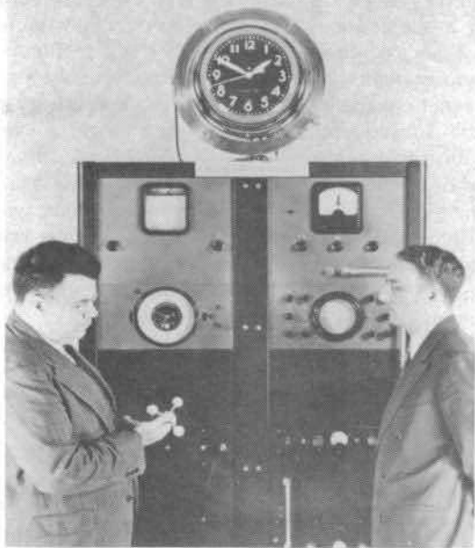
Fig. 4. E. U. Condon, H. Lyons, and the first atomic clock, Jan. 1949. Condon holds in his hands a model of the \text{NH}_3 molecule. Thirty feet of ammonia-filled, gold plated K-band waveguide, forming the absorption cell, are coiled around the electric clock at top; the absorption dip appears on the oscilloscope in front of Lyons. ("The atomic clock," NBS Tech. Rep. 1320, 1949; reprinted in J. Horological Inst. America , pp. 11–20, Feb. 1949, and pp. 7–14, Mar. 1949.)
