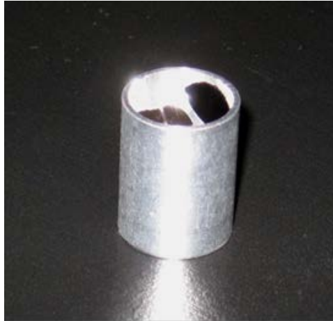
Figure 1: The 1/2" diameter retro-reflector used on STPSat-2
