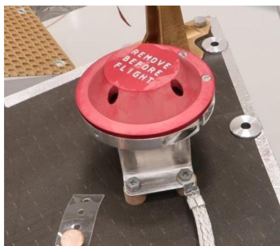
Figure 7-41. INRRI for ExoMars 2020 already installed on the top deck of the landing platform.
