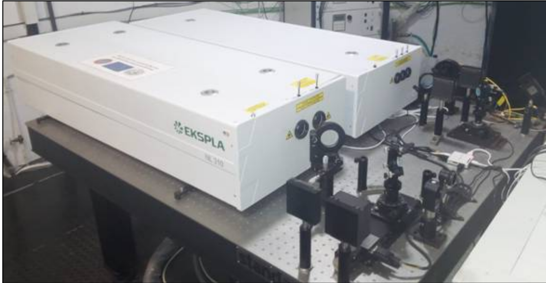
Figure 8-72. The laser bench installed at the San Fernando SLR station.
