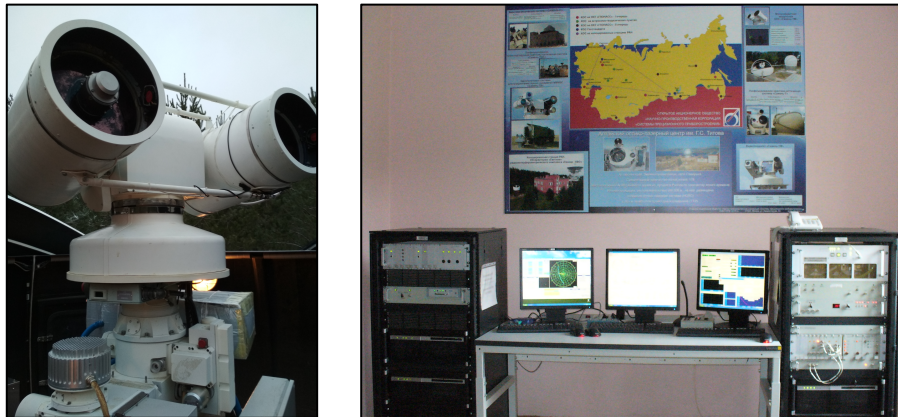
Figure 8-82. “Sazhen-TM” laser system (left) and the laboratory equipment of the system (right).
