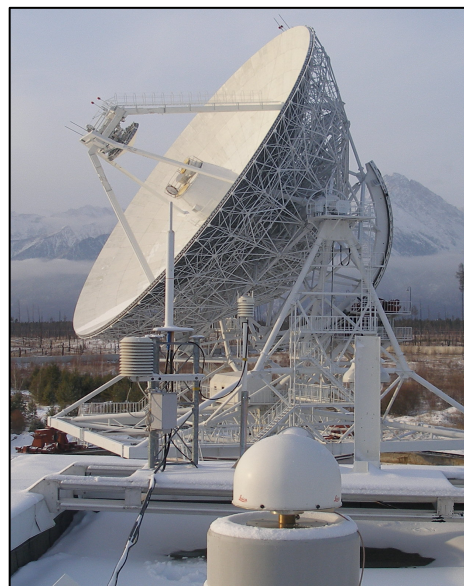
Figure 8-18. GNSS antenna, DORIS antenna and RT-32 radiotelescope.
