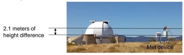
For example at Grasse, the met data in the CRD are corrected as follow: Pressure at the cross axes = pressure measured + 0.1176(hPa/m) x height difference (2.1m)
