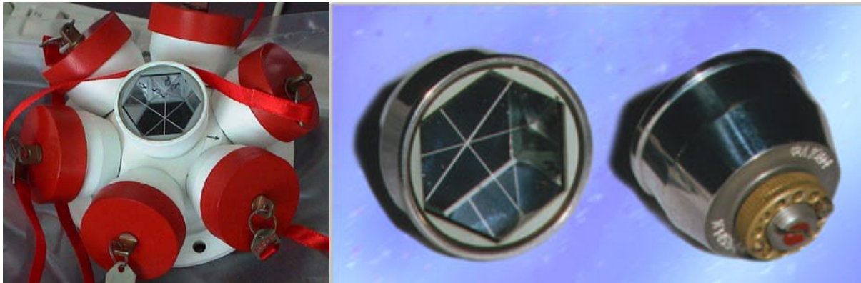
Fig. 1 IPIE laser retroreflector array for LEO satellites (left: GOCE flight model, right: individual prism). Images courtesy ESA and IPIE.
