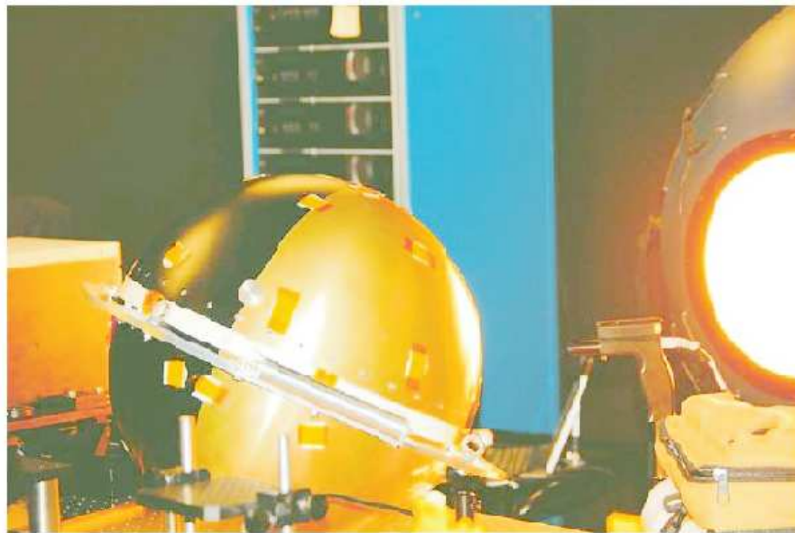
Figure 18: The spectral reflectance measurement setup for POLLUX.
