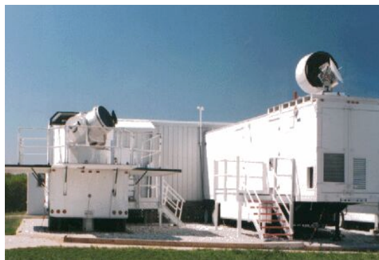
Figure 6 The NASA MOBILAS-5 SLR system in Greenbelt, Maryland; the aircraft RADAR is at top-right
