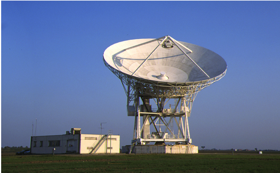
Figure 1. View of the Medicina 32 m dish taken during geodetic VLBI observations. Note that the subreflector is shifted to allow the use of the S/X receiver located in the primary focus of the radio telescope.
