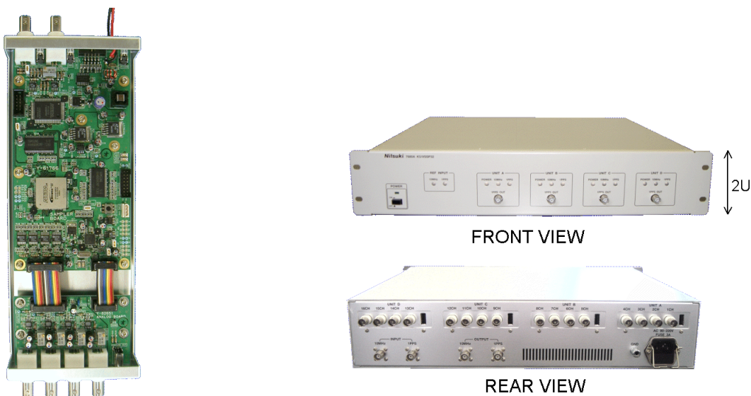
Figure 2. K5/VSSP32 unit (left) and 16 ch module (right).
