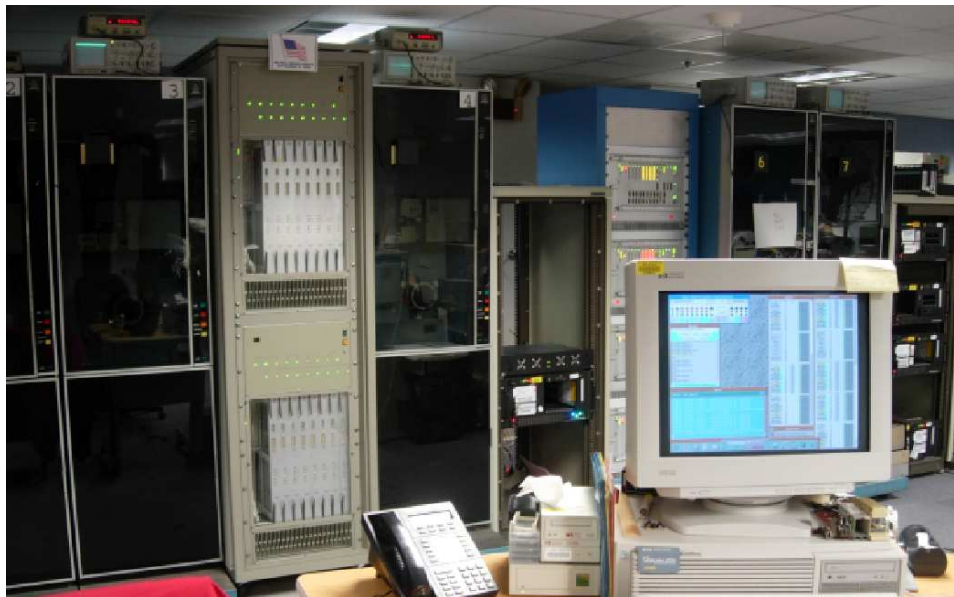
Figure 1. The right half of WACO showing 4 Mark 5A units (far right), legacy tape drives, the operator's console, Mark 5B (left of console) and the central processor (left).
