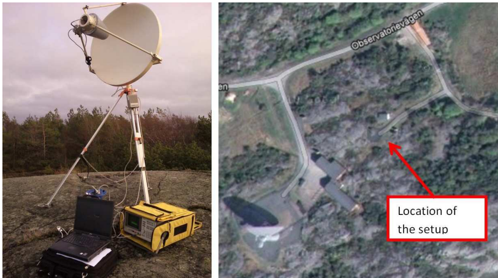
Figure 4. Left: setup for RFI-measurements. Right: map showing the location of the setup.
