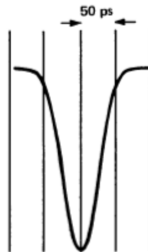
Figure 4a. Nd:YAG laser mode-locked pulse.
