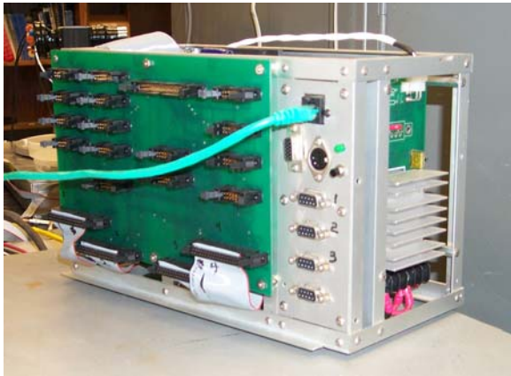
Figure 5: Front view of the Flight Control Unit (FCU)
