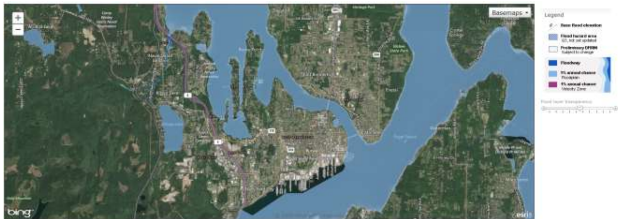
Figure B-4. FEMA Flood Insurance Maps for the 1% Annual Chance Floodplain for Bremerton (Flood insurance rate maps outline flood hazards in a community and includes flood insurance risk zones, 1% and 0.2% annual chance floodplains.)
