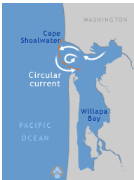
Figure 21: Cape Shoalwater Erosion Cycle
