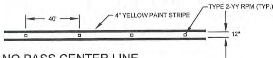
NO PASS CENTER LINE
