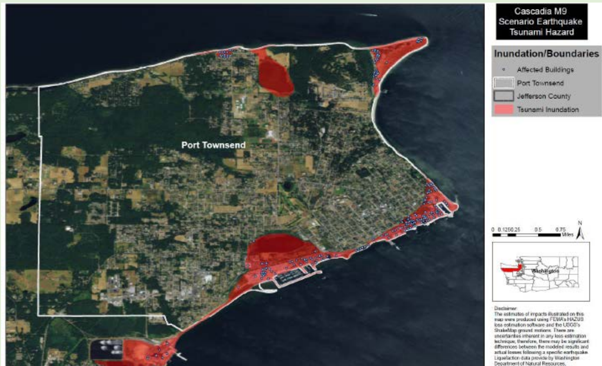
FIGURE TS-9 – PORT TOWNSEND BUILDING INUNDATION IN A SIMULATED CASCADIA M9 EARTHQUAKE-GENERATED TSUNAMI 22
