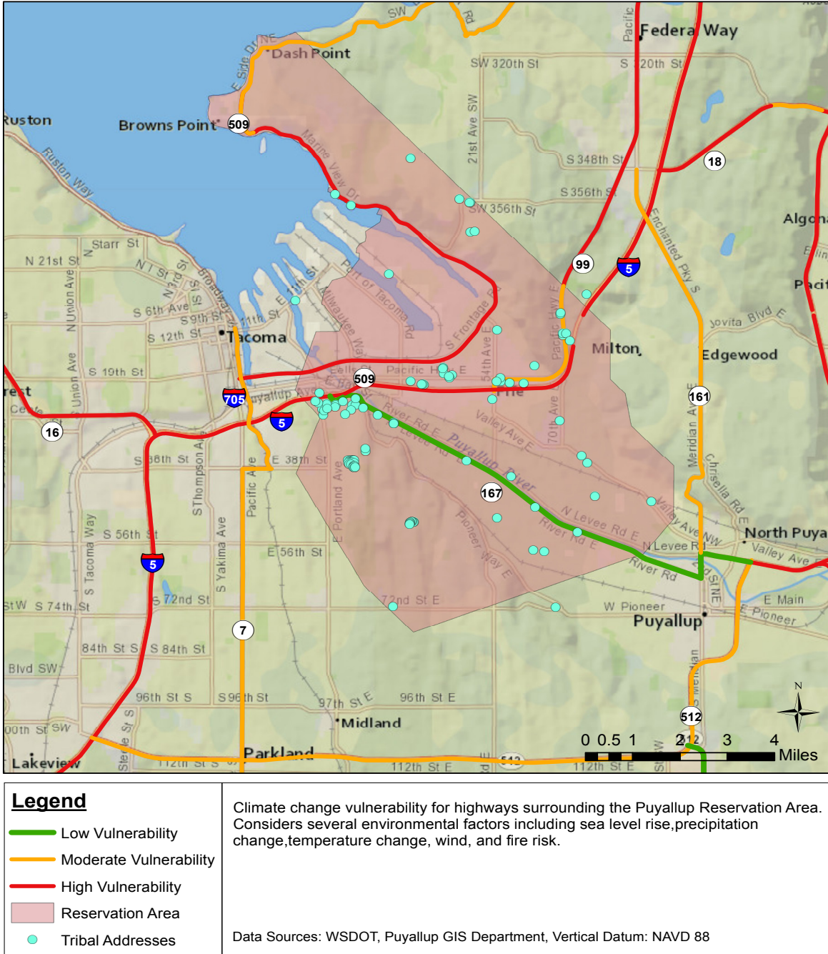
Figure 11. Vulnerability of Puyallup-area highways to one or more climate change impacts. Source: Washington State Department of Transportation 2011. [65]
