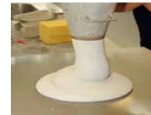
At compressive strengths above 150 Mpa one is no longer concerned with commonplace concrete. Stone aggregates are replaced for example by fine aggregates of ceramic origin, and the entire binder matrix is only slightly reminiscent of classical concrete. Shown in the illustration is the flow behavior of a UHPC of 200 MPa.
