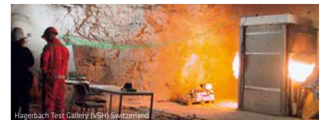
In special furnace chambers fire trajectories can be replicated, panels tested and subsequently evaluated. Temperature development is measured at various depths and recorded.
