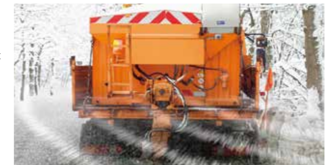
Scattered de-icing agent considerably intensifies the reaction upon freezing of water and leads to substantially greater damage in areas of concrete close to the surface.
