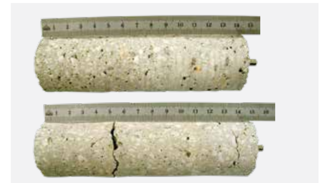
Concrete deterioration due to sulphate attack before & after the load shows a strong increase in length because of the spalling attack. First cracks have appeared in sample.
