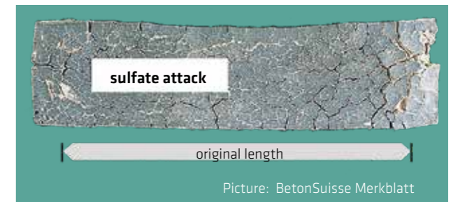
Sulfate driven attack is caused primarily by sulfates dissolved in water. By reacting with the hardened cement matrix, an increase in volume is induced which damages the structure.
