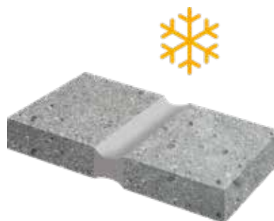
Contraction of building elements
