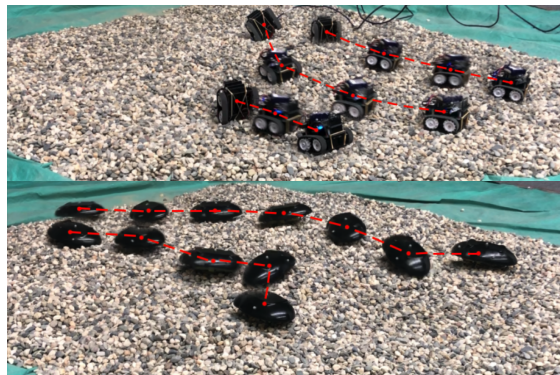
Fig. 4: Over 15 teleoperated trials performed on rough terrain, a legged robot succeeded in navigating through the terrain 90% of the time, whereas a wheeled robot of comparable size succeeded only 30% of the time.
