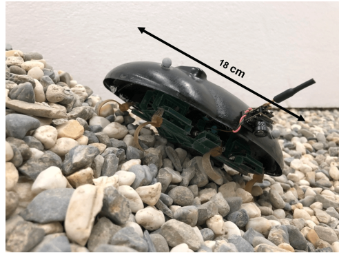
Fig. 1: VelociRoACH: the small, mobile, highly dynamic, and bio-inspired hexapedal millirobot used in this work, shown with a camera mounted for terrain imaging.
