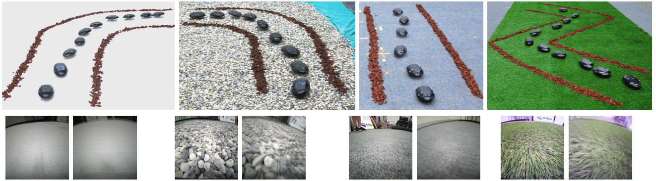
Fig. 5: Top: Execution of our model-based learning method, using an image-conditioned dynamics model, on various desired paths on the four terrains (styrofoam, gravel, carpet, and turf) we consider. Note that the path boundaries are outlined for visualization purposes only, and were not present during the experiments. Bottom: Example images from the onboard camera during the runs (shaky images due to body motion).
