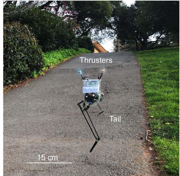
Fig. 1: Salto-1P jumps outdoors without external sensing.
