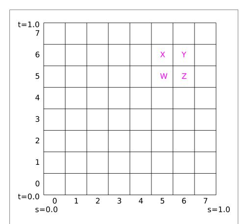
Figure 8.4. An example of an  $8\times 8$  texture image and the components returned for textureGather. The vector (X,Y,Z,W) is returned, where each component is taken from the post-swizzle component selected by comp of the corresponding texel.
