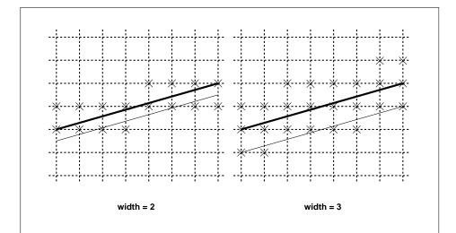
Figure 13.3. Rasterization of wide lines. x-major line segments are shown. The heavy line segment is the one specified to be rasterized; the light segment is the offset segment used for rasterization. x marks indicate the fragment centers produced by rasterization.
