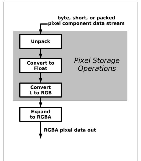
Figure 8.1. Transfer of pixel rectangles to the GL. Output is RGBA pixels. Depth and stencil pixel paths are not shown.
