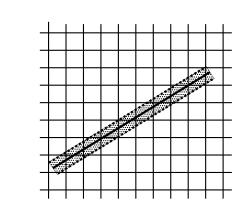
Figure 13.4. The region used in rasterizing a multisampled line segment (an x-major line segment is shown).
