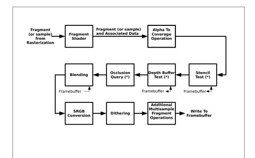
Figure 15.1. Per-fragment operations. The boxes labelled with "(\*)" may instead be performed during early per-fragment operations, as described in section 13.6.
