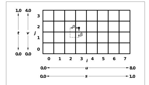
Figure 8.3. A texture image and the coordinates used to access it. This is a two-dimensional texture with *width* 8 and *height* 4.  $\alpha$  and  $\beta$ , values used in blending adjacent texels to obtain a texture value are also shown.
