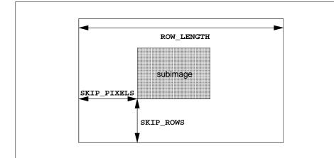
Figure 8.2. Selecting a subimage from an image. The indicated parameter names are prefixed by UNPACK\_ **TexImage\*** and by PACK\_ for **ReadPixels**.
