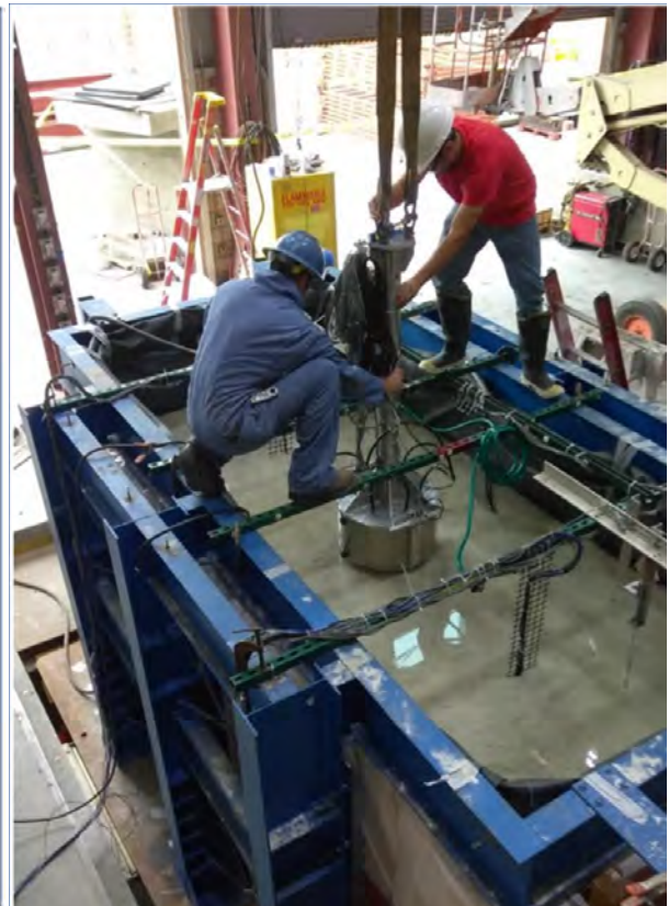
Figure 2. Deployment of the bucket in the saturated soil with lower part of the tower.
