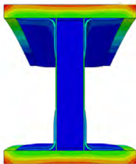
Figure 1. Finite element simulation of an aircraft's composite wing spar.
