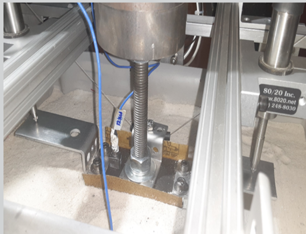
Figure 1. (left) Model footing on the shake table in the UC San Diego centrifuge. Figure 2. (right) Footing response without ground improvement (a) and with paired cement-mixed columns (b). Note that footing (b) exhibits greater moment capacity, reduced settlement, and improved re-centering.
