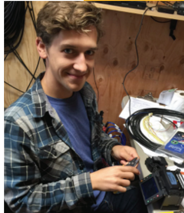
Figure 3 Nate Lindsey making an arc fusion splice.
