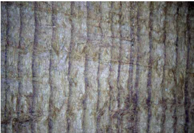
Figure 11: Fiber of ASM 12496 deformed under pressure of wood-working tools. Photograph courtesy of Tomasz Wazny.
