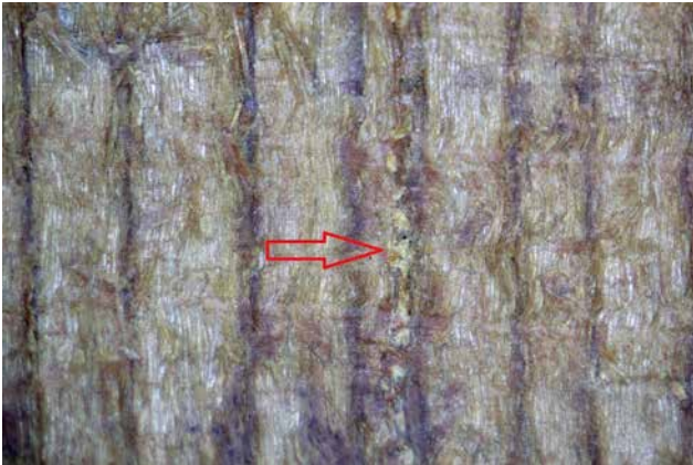
Figure 9: Traumatic resin canals visible on the radial surface of board. Photograph courtesy of Tomasz Wazny.
