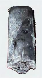
Third-party battery after an External Short-Circuit test, which is intended to simulate an unintended circuit fault.
