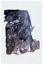
Third-party battery after an Abusive Overcharge test, which is intended to simulate charging the battery beyond its intended limits.
