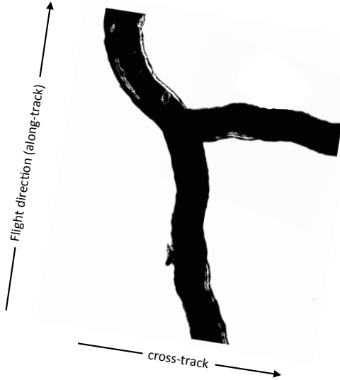
Figure 70. Illustration of the two cases considered for high frequency slope errors for a river (represented by the black surface), where one reach is aligned in the flight direction and the other one perpendicular to it.
