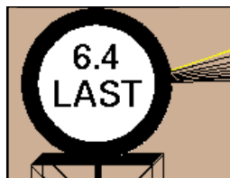
Figure 4. LAST on the radome used to indicate the final elevation.
