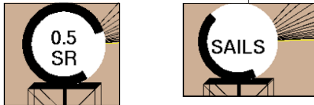
Figure 1. First 0.5 scan (left) and SAILS scan (right) indicators on the radome at the RPG HCI.
