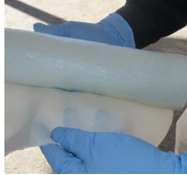
SikaWrap® PreSaturated 100G glass fabric being unrolled
