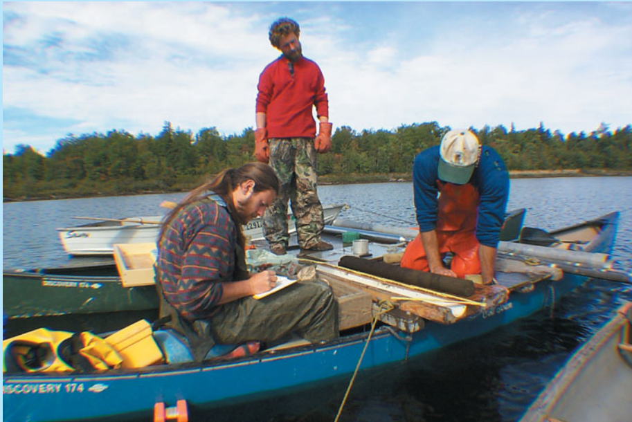
Geologists recording and preparing a lake sediment core for transport to the laboratory for detailed analysis.
