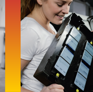
Each drivetest vehicle carried nine smartphones for the voice and data tests.
