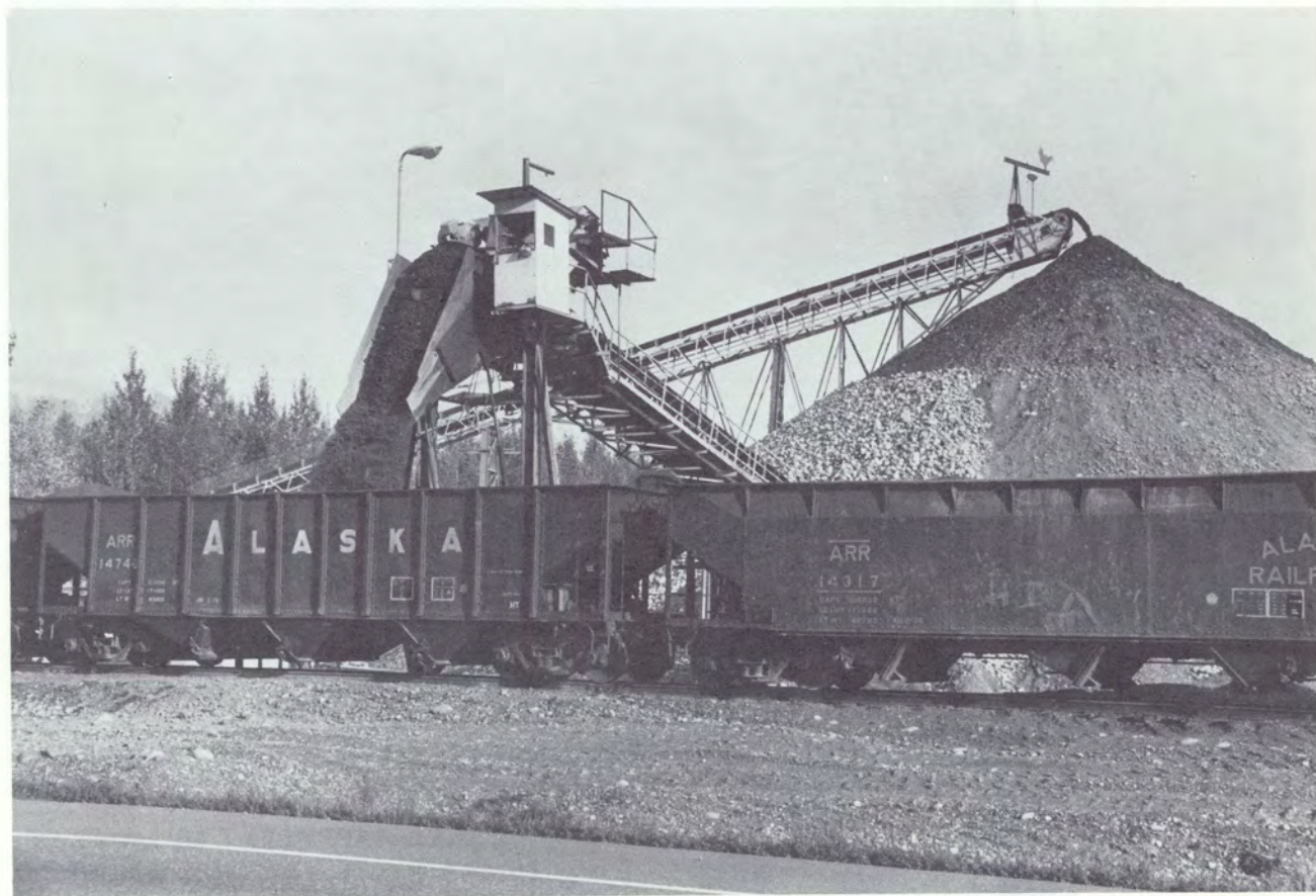
Loading unit train carrying gravel, in Palmer. Operating four 80-car trains per day during the summer, the Railroad hauled 2.75 million tons in FY 1982.
