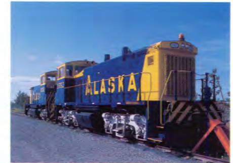
Two 1,500-horsepower switch engines were purchased in 1992 to free road engines for heavier work and to improve customer service.
