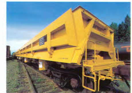
Twenty-seven 100-ton side air-dump cars were purchased to haul track maintenance materials but also can be used in freight service to haul natural resources such as gravel.
