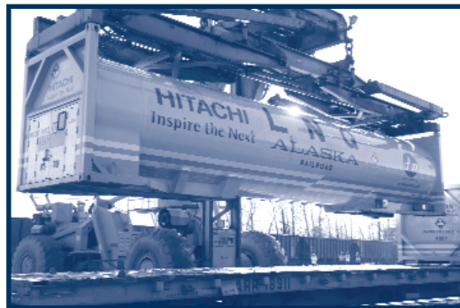
An LNG-filled ISO container is loaded onto a flatcar before being added to a northbound freight train.
