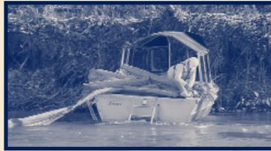
*Fast water boom is deployed to confine the simulated oil spill.*
