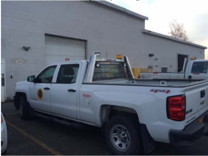
Truck bed ladder rack – 1,000 lbs. minimum weight capacity required
