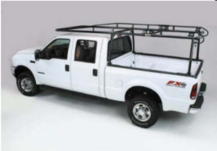
Truck bed ladder rack – 1,000 lbs. minimum weight capacity required
