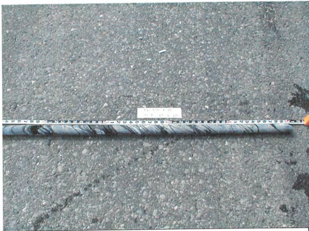
Abutment 5, TH 19 rock core from 9.45 m to 10.97 m in depth.
