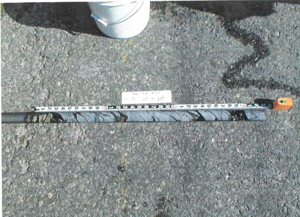
Abutment 5, TH 20 rock core from 6.1 m to 7.01 m in depth.
