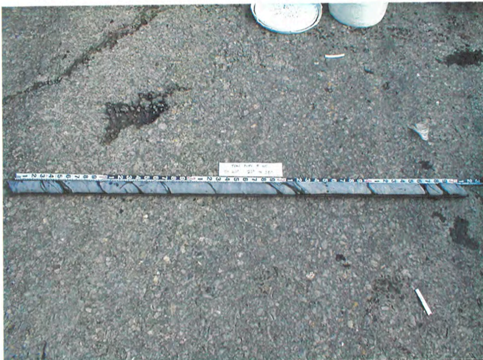
Abutment 5, TH 20 rock core from 7.62 m to 9.14 m in depth.
