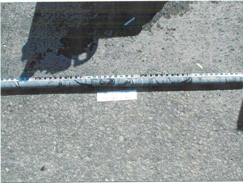
Abutment 5, TH 20 rock core from 10.37 m to 12.19 m in depth.
