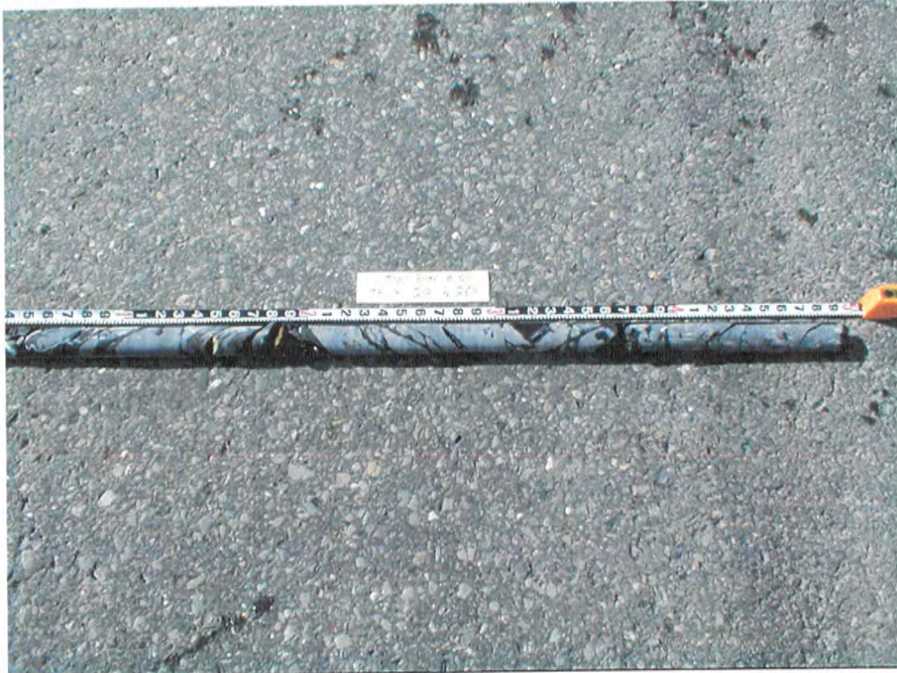
Abutment 5, TH 19 rock core from 7.92 m to 9.45 m in depth.
