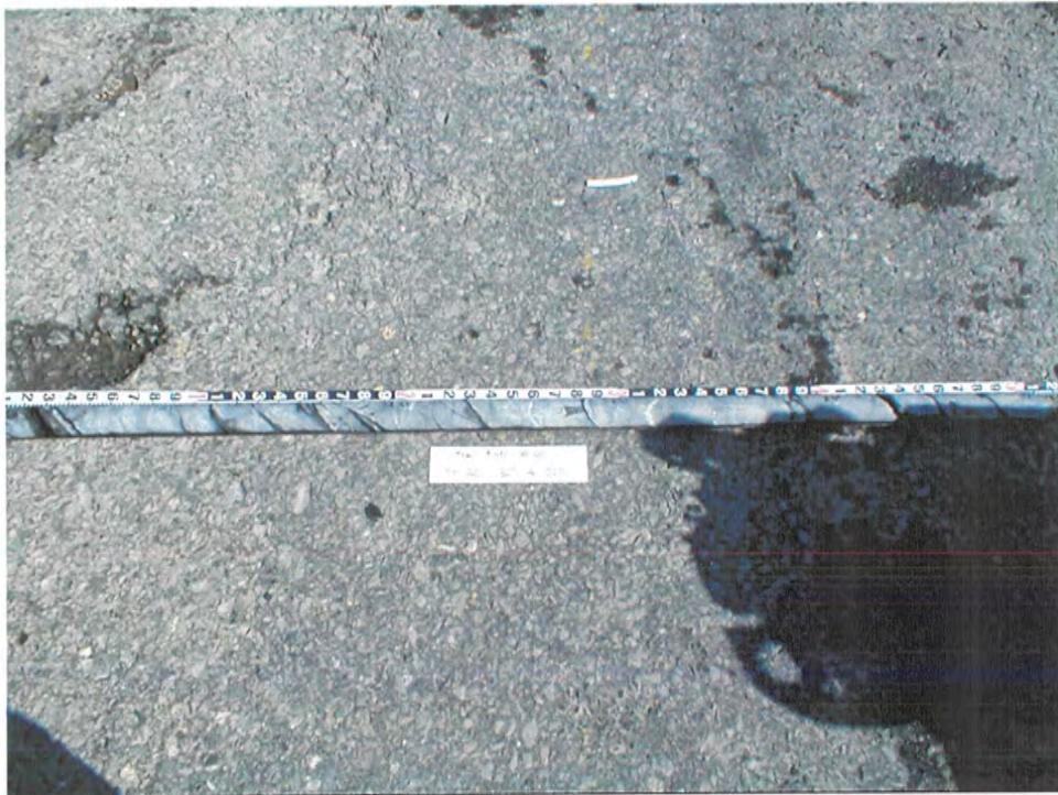
Abutment 5, TH 20 rock core from 9.14 m to 10.67 m in depth.
