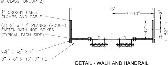
EVERY 4th TIE TO BE 8" x 8" x 16'-0" FOR WALKWAY AND HANDRAIL SCALE: 3/16" = 1'-0"
