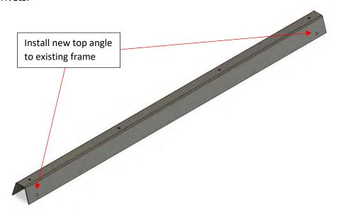
5. Install new frame divider rail, PN ARR-45X-0006 using (4) #6x2" SS sheet metal screws installed from under side:
