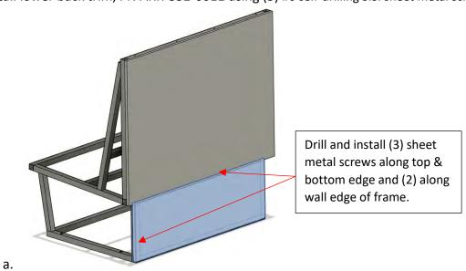
3. Install lower side trim, PN ARR-352-0001 using (6) #6 self-drilling S.S. sheet metal screws:
