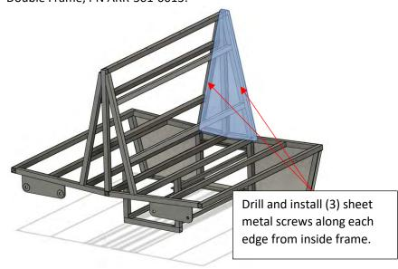
4. Install divider rail, PN ARR-301-0010 using (4) #6x2" SS sheet metal screws installed from under side. Note, single frame shown, double frame uses PN ARR-301-0011:
