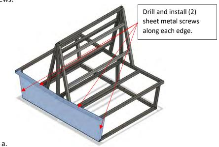
2. Install side trim board, PN ARR-352-0013 using (6), #6x 1.25" S.S. dome head sheet metal screws:
