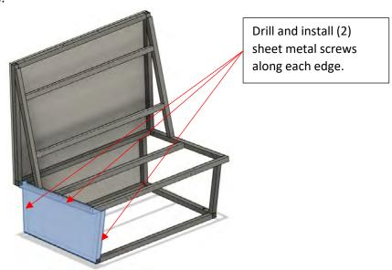
4. Install side trim board, PN ARR-352-0012 using (6), #6x 1.25" S.S. dome head sheet metal screws:
