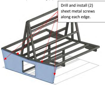
3. Install upper frame side trim PN ARR-301-0012 using (6), #6x 1.25" S.S. dome head sheet metal screws:
