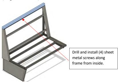
5. Assemble and install double seat frame drawer (PN ARR-301-), drawer face (PN ARR-301-) and latch using (4) machine screws, washers and nuts:
