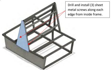
3. Install divider rail, PN ARR-352-0009 using (4) #6x2" SS sheet metal screws installed from under side:
