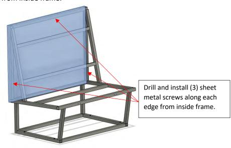
2. Install lower back trim, PN ARR-352-0011 using (5) #6 self-drilling S.S. sheet metal screws:
