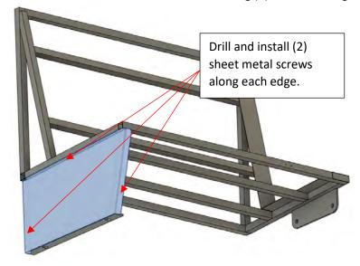
Double frame (install using (8) screws):
