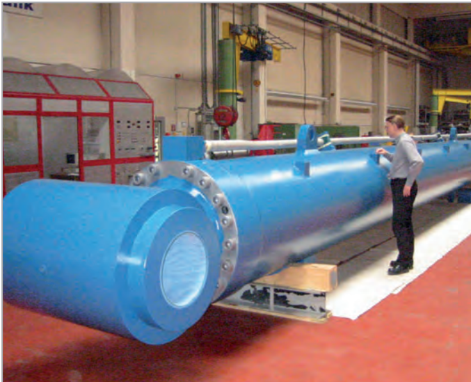
Piling barge cylinder with 900 mm piston diameter
