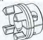
Design 2.1 clamping hub, single slit, with keyway
