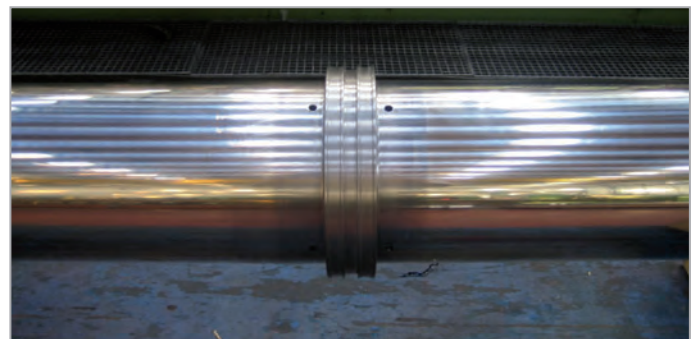
Double piston rod with centred piston, Ultraplate coating and oil feeding through the rod
