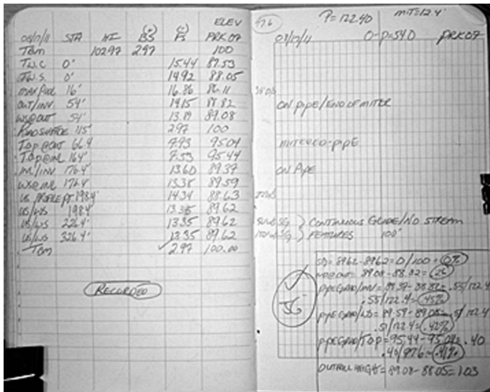
Figure 45.—Sample of survey data and calculation in a field notebook.
