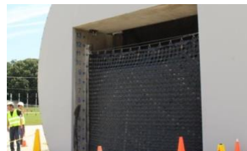
12' TALL X 16' WIDE SIDE DEPLOYED FLEX-WALL TESTED AT 10 FT. OF WATER
