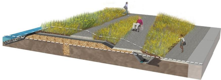
Graphic rendering of cross-section of incremental vegetated berm option presented in Section 4.0 Sample Vegetated Berm Barrier.
